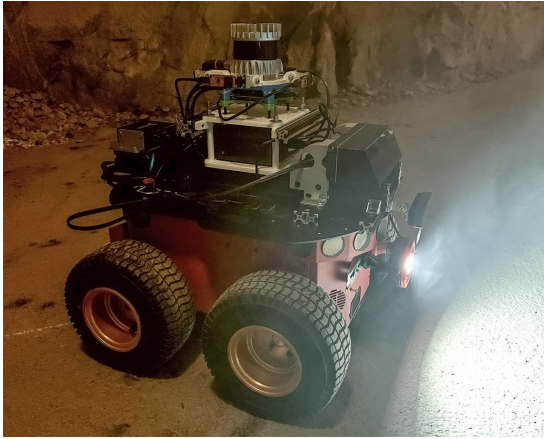
(a) Pioneer 3-AT2 mobile base carrying the sensor tower. The four-wheel, skid-steered platform supports up to 30 kg payload and can negotiate rough terrain—providing the mobility required for subterranean data collection.
